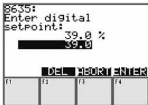
Entry mask for the digital input value.
