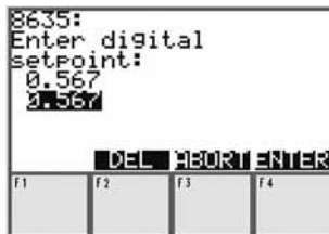
Entry mask for specifying a setpoint step.
